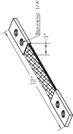
**CONECTOR DE COBRE TRENZADO FLEXIBLE TIPO BD**
