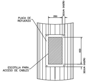
**DETALLE DE VENTANAS INFERIORES V1', V2'**
